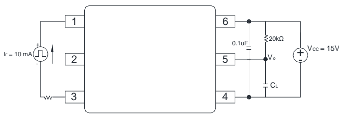
Figure 5 : Propagation Delay Test Circuit.
