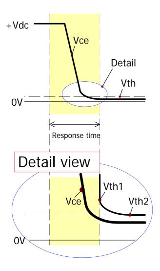
Fig. 5 Collector-sense voltage curve
