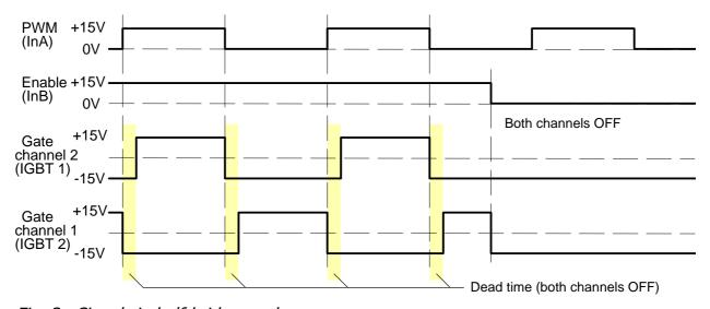
Fig. 3 Signals in half-bridge mode
