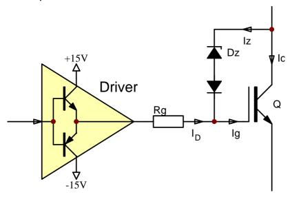
Fig. 10 Basic circuitry for active clamping
