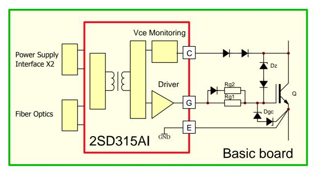
Fig. 2 Separation of universal (red) and IGBT-specific functions (green)
