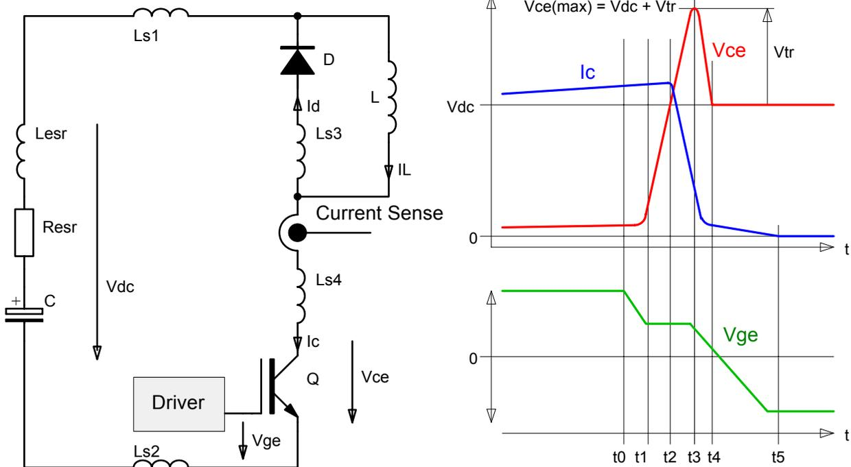
Fig. 9 Test circuit (left) and typical switching behavior (right)
