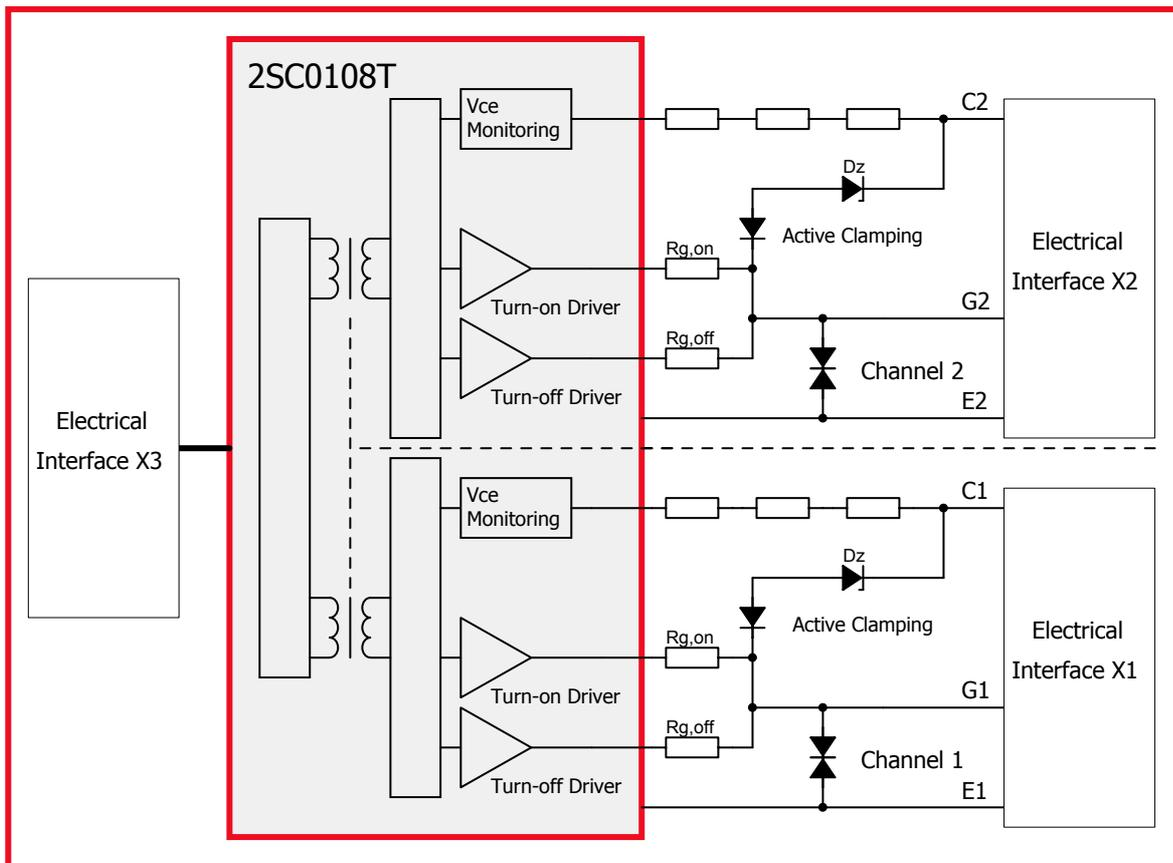
Fig. 2 Basic schematic of the 2BB0108T basic board with 2SC0108T driver
