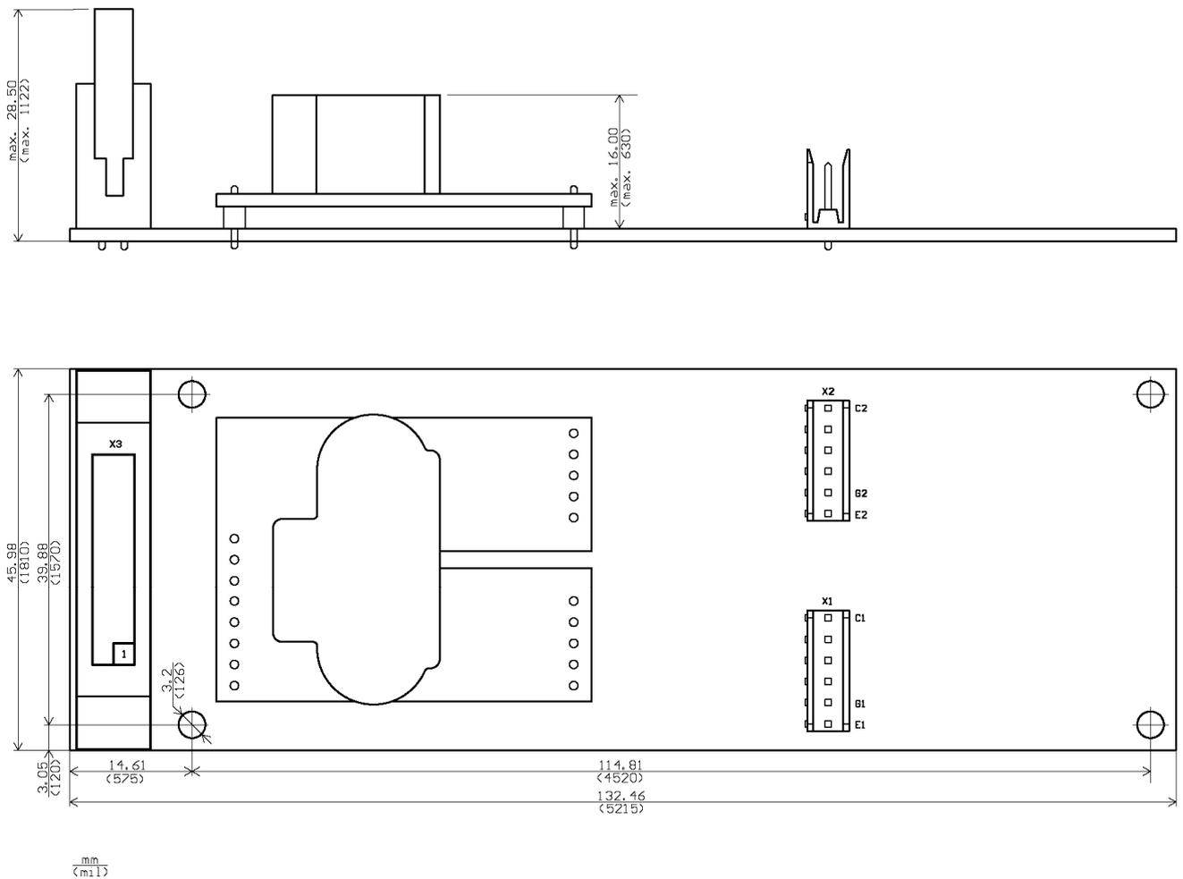
Electrical connector on the basic board: 71918-120LF from FCI
