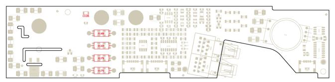
Fig. 1: Assembly drawing of 1SP0635x2Mx with highlighted gate resistors
