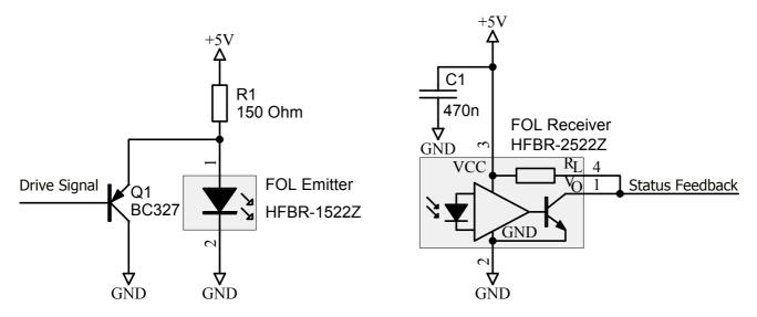
Fig. 12 Recommended circuitry for the "versatile" fiber-optic links (1SP0635V)
