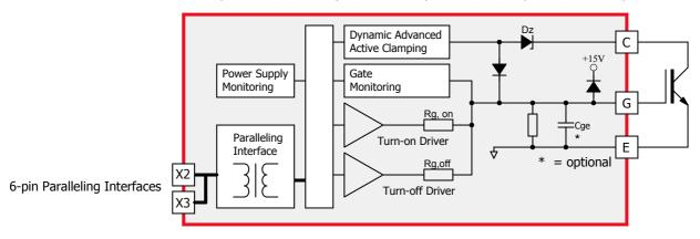
Fig. 3 Basic schematic of the 1SP0635D drivers
