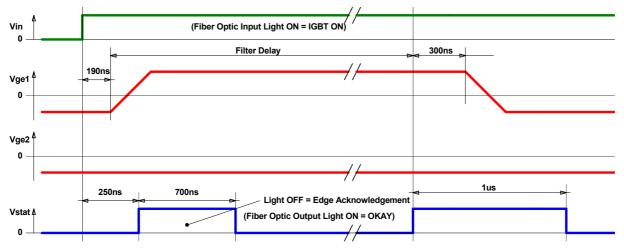
Fig. 10 Driver behavior and status feedback in the event of a gate-monitoring fault at turn-on
