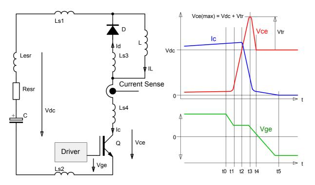
Fig. 17 Test circuit (left) and typical switching behavior (right)
