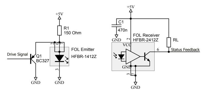
Fig. 13 Recommended circuitry for the "ST" fiber-optic links (1SP0635S)
