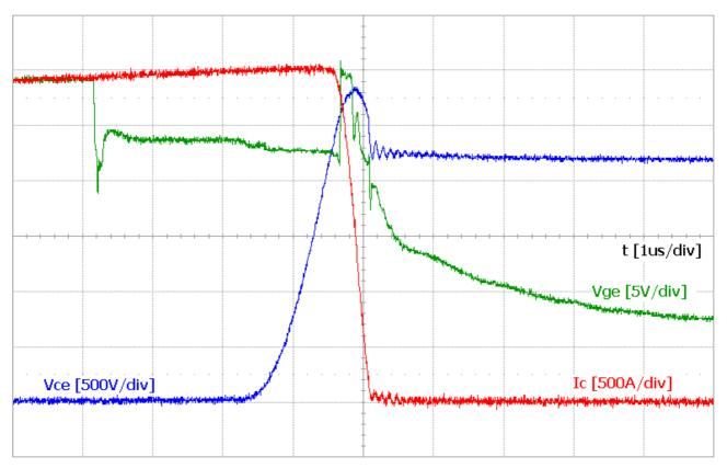
Fig. 18 Behavior of a 1500A/3300V IGBT module turning off at a DC-link voltage of 2200V a collector current of 3000A, which is twice the nominal collector current
