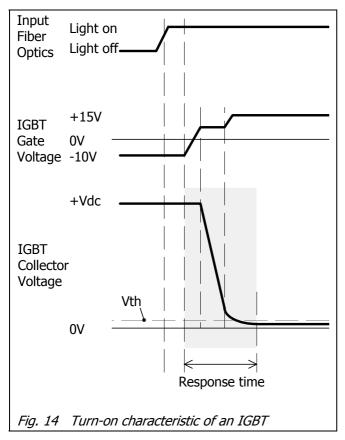
A dynamic  $V_{\text{ce}}$  monitoring circuit is implemented in 1SP0635V and 1SP0635S gate drivers. The IGBT collector-emitter voltage is measured with a resistor network.
