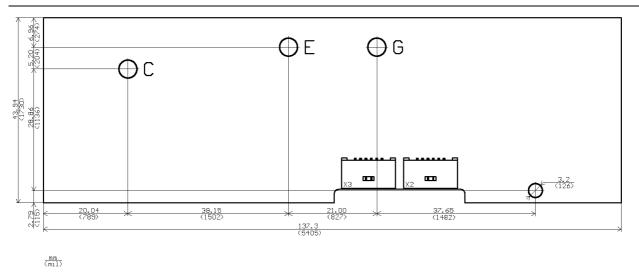
Maximum driver height: 6mm measured from the bottom layer
