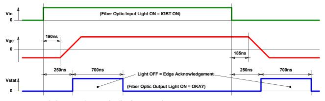
Fig. 8 Driver behavior and status feedback in normal operation
