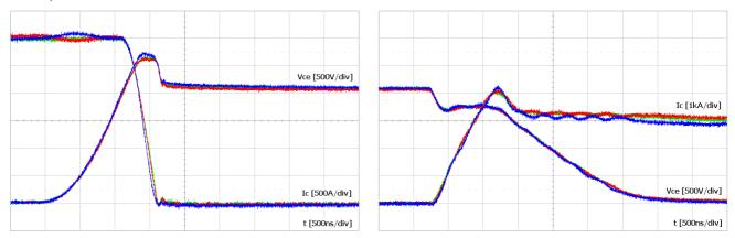
Fig. 16 Turn-off (left) and turn-on (right) behavior of three 1500A/3300V IGBT modules in parallel connection at a DC-link voltage of 2200V and a collector current of 3000A each
