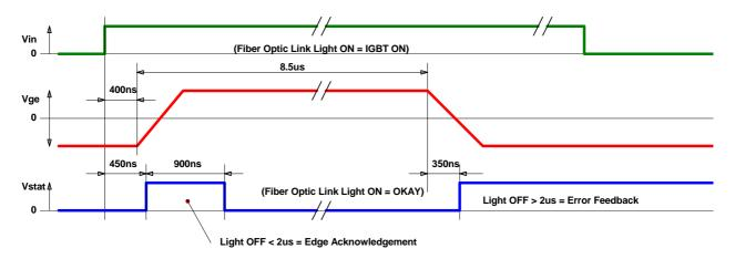
Fig. 12 Failure status feedback; signals under short-circuit conditions in 2-level mode
