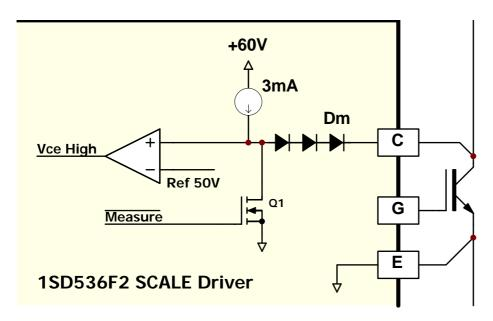
Fig. 4 V<sub>ce</sub> desaturation monitoring
