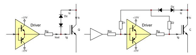
Fig. 6 Basic active clamping circuitry (left) and advanced circuitry used in 1SD536F2 plug-and-play drivers (right)
