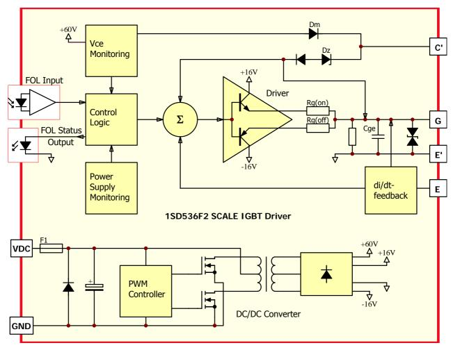
Fig. 3 Block diagram of the 1SD536F2 SCALE driver
