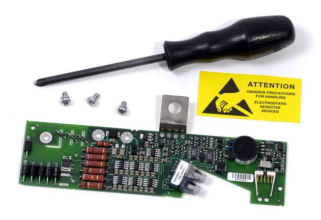
Fig. 2 SCALE plug-and-play driver and the required tool
