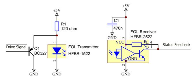
Fig. 14 Recommended circuitry for the fiber-optic links (standard version)
