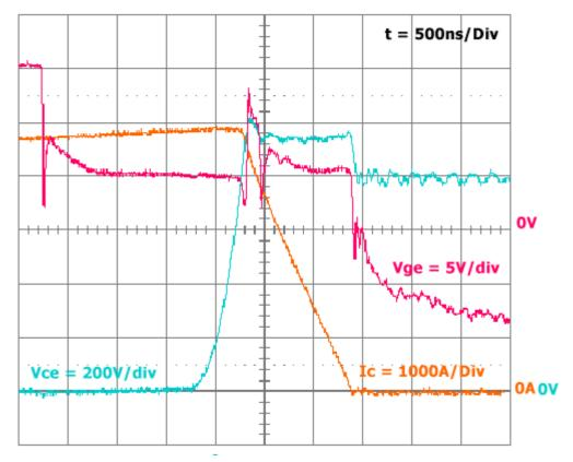
Fig. 7 Behavior of a 2400A/1200V-IGBT for turning off a collector current of 4800A, which is twice the nominal collector current
