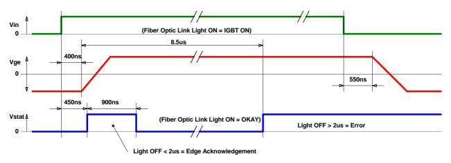
Fig. 13 Failure status feedback; signals under short-circuit conditions in 3-level mode
