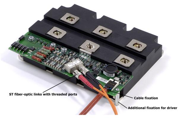
Fig. 17 Additional measures for fixing driver and power-supply cables as well as the ST optical fiber with a threaded port (Opt. 1)
