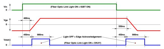
Fig. 11 Failure status feedback; signals for normal operation
