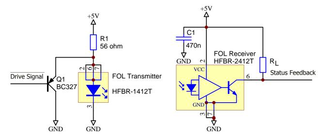
Fig. 15 Recommended circuitry for the fiber-optic links (Opt. 1)
